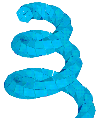
A spiral well is an example of a grid formed along an arbitrary well path.
